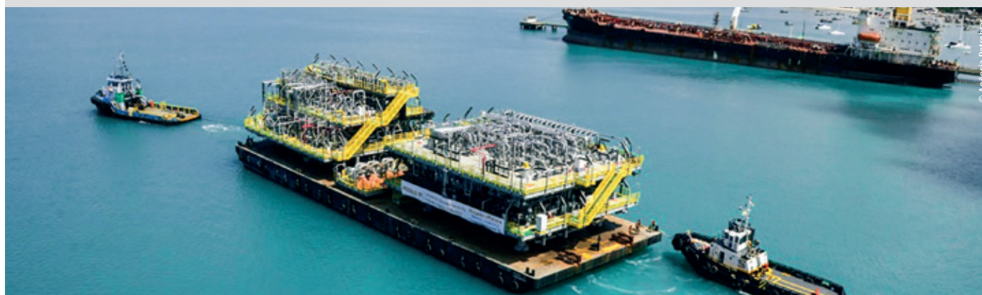
OIL PROCESSING MODULE TRANSPORT FOR REPLICANT FPSO
